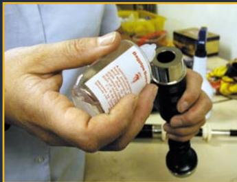
2. Always check that all hemping is secure. Joints should be airtight but not solid. Tuning should be easily done with one hand but tight enough to prevent the top from slipping.
