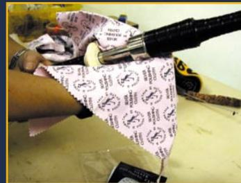
4. Metal parts should be polished with a soft dry cloth. Ideally a silver cloth is recommended. NEVER use any abrasive cleaners on plated parts. This may damage the plating and void your guarantee.
